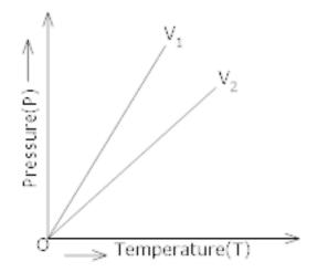
For a given temperature,  $P\alpha \frac{1}{V}$  therefore when the gas is heated in a small vessel (Volume  $V_1$ ), the pressure will increases more rapidly than when heated in a large vessel (Volume  $V_2$ ). As a result, the slope of P – T graph will be more in case of small vessel than that of large vessel.
